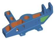
Horizontal area and horizontal core machining both have similar smoothing characteristics to area clearance and can detect all flat surfaces on a part, with or without using boundaries.
