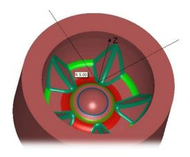
A draft function shows draft angles (tapers from the tool axis) using a similar style of graphical display as the curvature.
