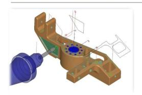
3+2 multi-axis machining has an easy to use graphical interface, including being able to snap to the surface normal for machining.
