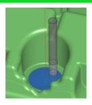
This creates an archimedean spiral toolpath from a given focal point, generating a constant contact as it machines within a given boundary. It is ideally suited for use on round shallow areas using contact angles between  $0^{\circ} - 30^{\circ}$ , in conjunction with the waterline machining for the more vertical faces  $30^{\circ} - 90^{\circ}$ . These passes can be constrained to a boundary or by the selected surfaces.
