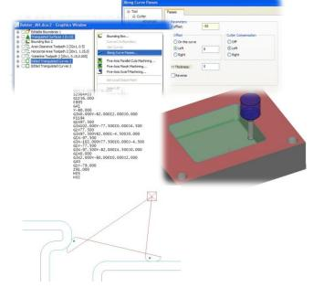
The optional pass overlap allows the cutter to overlap the starting position (closed profiles) to help reduce a 'tool line', giving a better surface finish.
