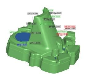
**NCG CAM** has an inspection module which allows the machined part to be inspected while still on the CNC machine tool.
