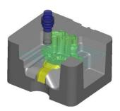
**NCG CAM**'s automatic roughing of surface data is suitable for all types of 2D or 3D forms, creating an optimised, smooth cutting motion for high speed machining (HSM) while maintaining part accuracy, cutting tool life and machine tool life. All cutters and tool-holders are collision protected to maximise efficiency and stock model visualisation of the machined part is available at every stage of the manufacturing process.
