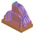
Rest roughing can also be used when machining castings. The passes can be trimmed back to another surface model such as the casting form seen below. The resultant rest toolpath is fast to create and cuts out multiple tooling operations, fresh air cutting and set-up time.
